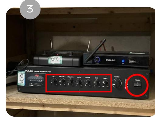
3 Switch on amplifier and adjust volume for required input.
